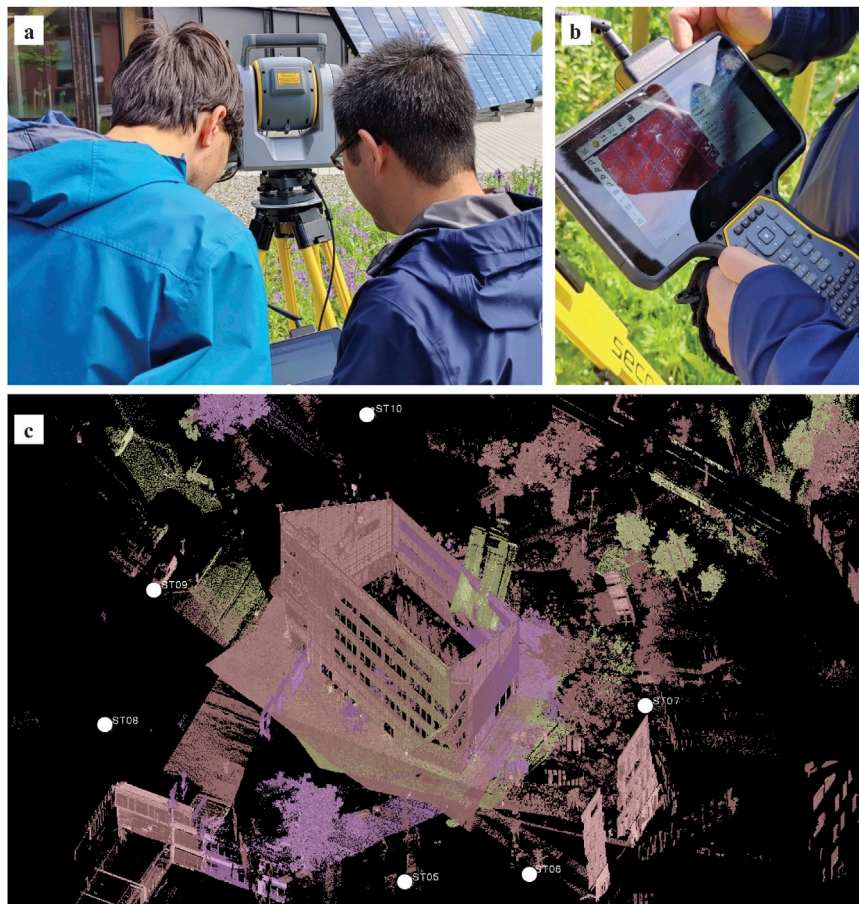
FIGURE 5 From the top: (A) scanning operations, (B) view of the point cloud during the scanning operations, and (C) positions of scanning stations around the ZEB Laboratory.
