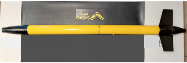
Figure 3. OASYS underwater glider (Elkolali et al. (2022)), courtesy of OsloMet
