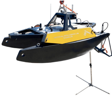
Figure 2. Maritime Robotics Otter USV with Waterlinked short-baseline (SBL) acoustic antenna/receivers, courtesy of OsloMet
