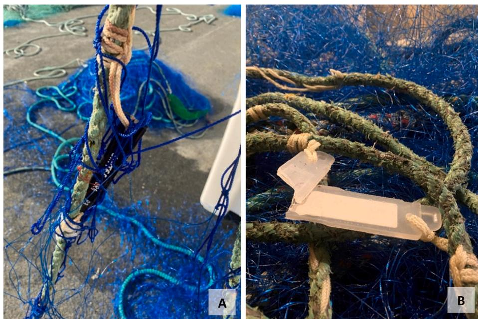
Fig. 6. Tag-A entangled in the net (A) and a broken Tag-B, tightly tied to the rope (B).
