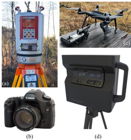
Figure 2 – Data acquisition equipment: (a) Terrestrial laser scanning; (b) Canon EOS 5D; (c) Unmanned aerial vehicle – 3DR SiteScan; and (d) Infrared scanning – Matterport Pro2 3D.
