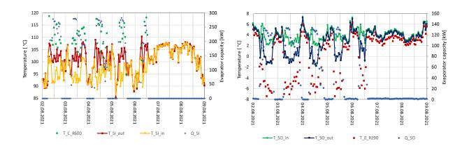
Figure 4: HTHP operation: a) R600 Condenser characteristics, b) R290 evaporator characteristics
