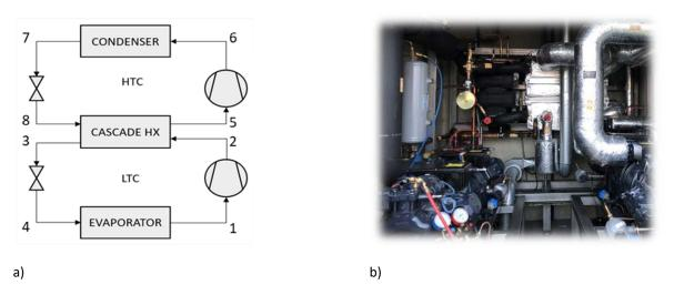
Figure 1: Industrial HTHP a) simplified cycle scheme, b) picture of installed prototype
