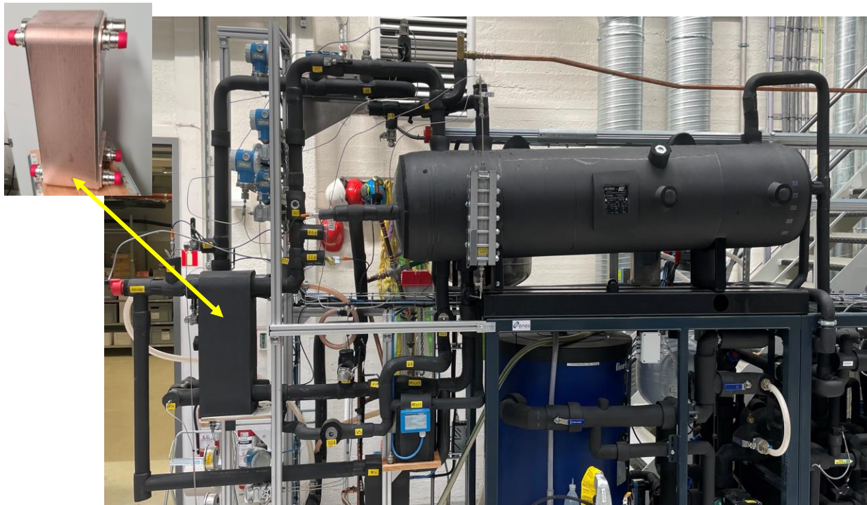
Figure 2: Picture of the CO 2 facility at NTNU/SINTEF with the two-stage evaporator on the lower left-hand side.
