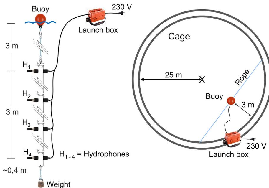
**Fig. 1.** Hydrophone array configuration and rig placement in the fish cage in Case 2 and Case 3. Case 1 used the same rig, but with only a single hydrophone placed in position H<sub>4</sub>. The rig was then placed in the net-pen in the same way as for Cases 2 and 3. The circumference of the fish cages was 157 m (radius of 25 m). The net consisted of vertical cylindrical wall and a conical bottom.
