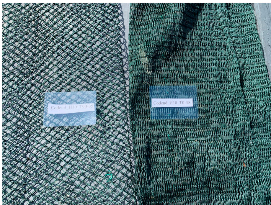
Figure 8. The mesh opening of the T90_35 (left) and T0_35 codend (right) in natural conditions after experimental fishing.
