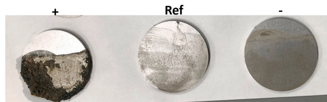
Fig. 8. Photography of steel electrodes: anode (+), cathode (-) and the reference surface (Ref) after removal from the cement dispersion in water.
