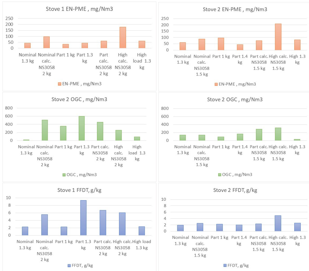
Figure 8: Results of different fuels loads and heat outputs when tested in accordance with EN16510-1 and PM EN-PME, OGC with parallel sampling in the full flow dilution tunnel in accordance with NS3058 and calculating in g/kg
