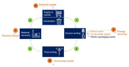
Figure 2: Representative plastic packaging value chain showing main units and streams with plastic packaging.
