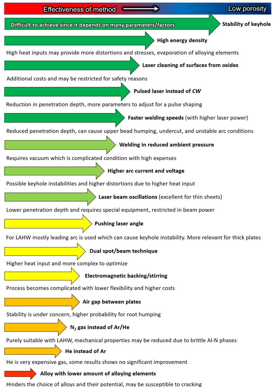
Figure 20. Porosity mitigation mechanisms in LBW/LAHW. Note, ranking is based on effectiveness, costs, and practical use in industry. Below the arrows, the reasons of low overall effectiveness and disadvantages are presented.
