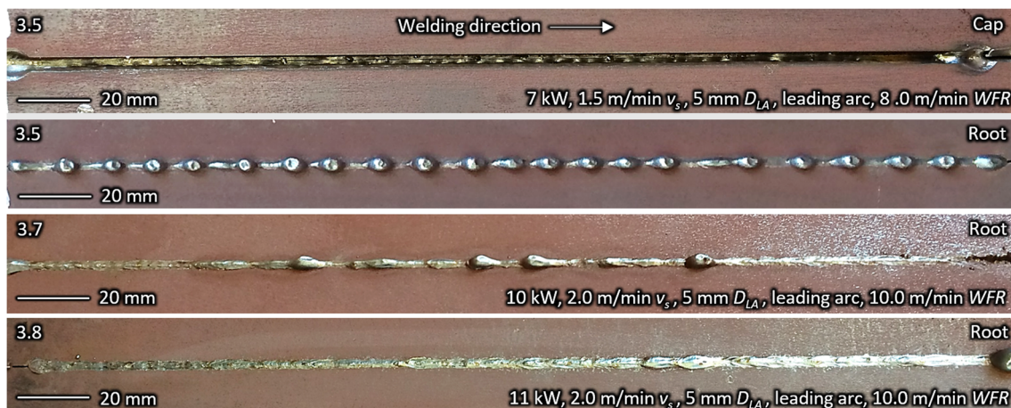
Fig. 12 Appearances of Weld No. 3.5, 3.7, and 3.8. Constant parameters: FPP = 0 mm and 0.4 mm air gap
