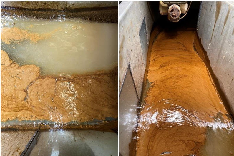
Figure 4-9 Emulsion 30 minutes after the third application of Dasic Slickgone NS
