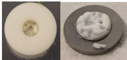
Fig. 2. Deposits on carbon steel specimen inside holder (left) and when removed from holder (right). TCD was 200 A/m 2 at 50 Hz.
