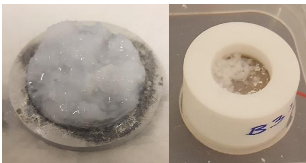
Fig. 5. Deposits on aluminum specimen at TCD of 80 A/m 2 at 50 Hz (left) and TCD of 40 A/m 2 at 200 Hz (right).
