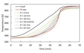
Figure 4 Simulations results. Fluid temperature in center of fuel bed at different elevations
