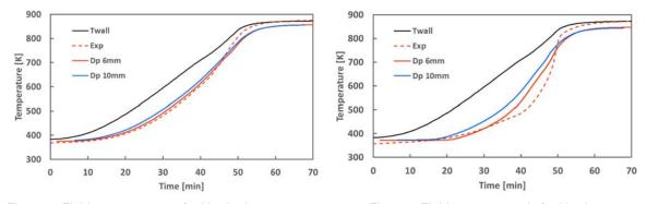
Figure 5. Fluid temperature at fuel bed edge at different particle diameters (Dp)
