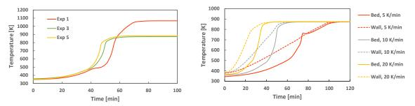
Figure 3: Left: The temperature profile during heat-up in the center of the pellets bed for experiments 1, 3 and 5, **Right**: The temperature profile during heat-up at the reactor wall and in the center of the fuel bed for experiments 2, 3 and 4 with heating rate 20, 10 and 5 K/min, respectively
