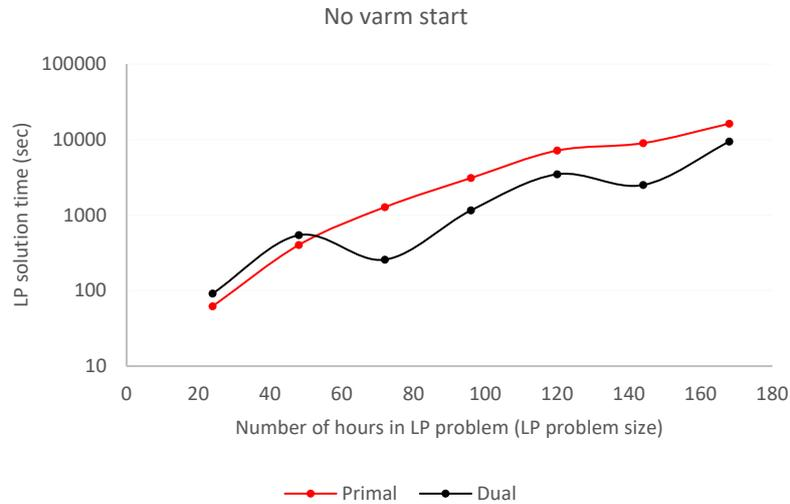
**Figure 5: The LP solution time without warm start for varying LP-problem size. The black curve shows the results from the Dual Simplex method and the red curve shows the results from the Primal Simplex method. The vertical axis has a logarithmic scale.**
