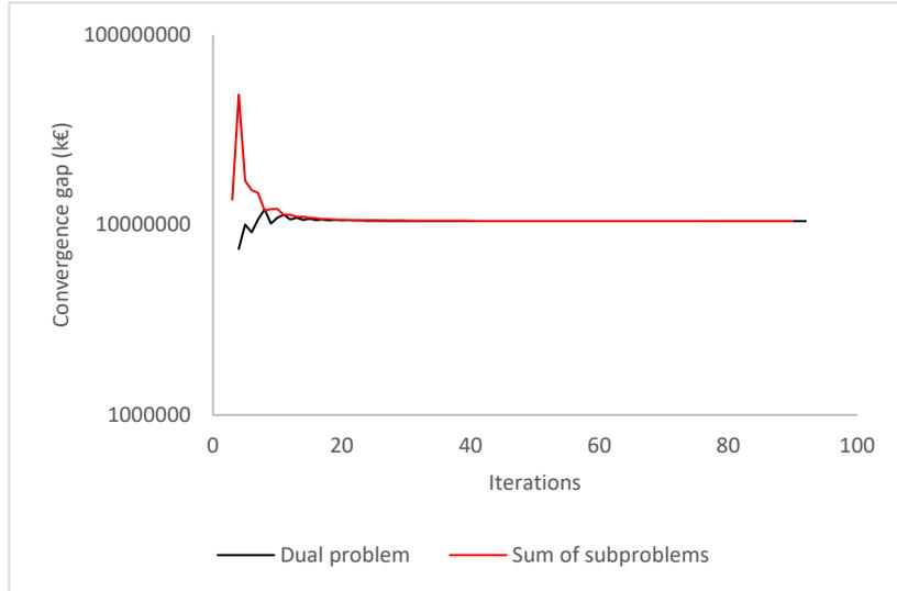
**Figure 37: The evolution of the convergence gap of the LR solution process for parameter values from configuration 2.**
