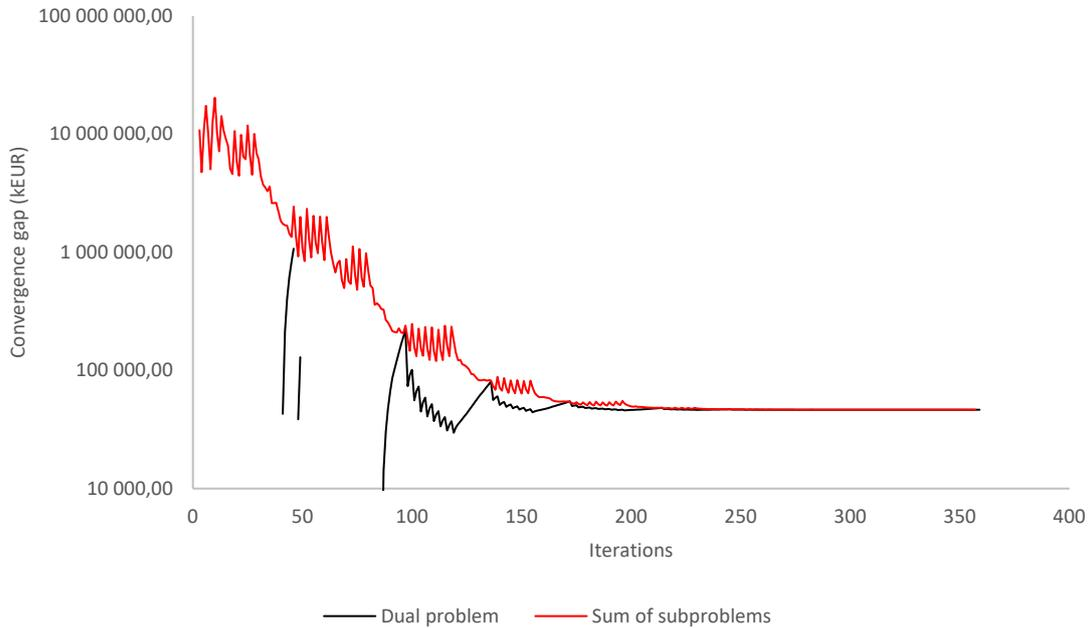
**Figure 18: The convergence gap versus the iteration number of the LR iteration process.**
