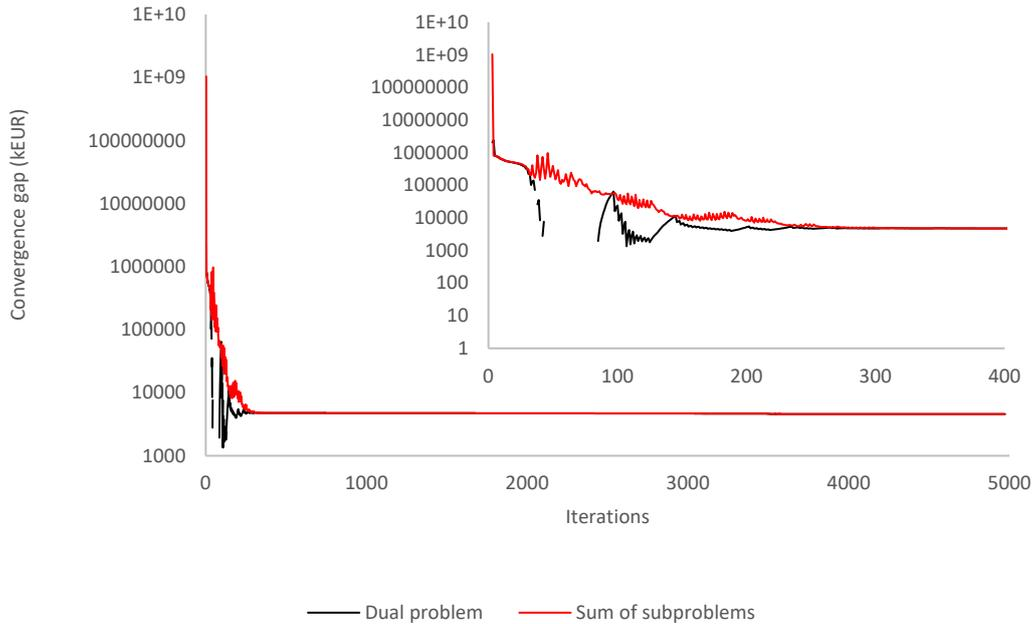
**Figure 7: The evolution of the convergence gap for the dual problem and the LR per iteration. The embedded figure shows the evolution of the convergence gap for the first 400 iterations.**
