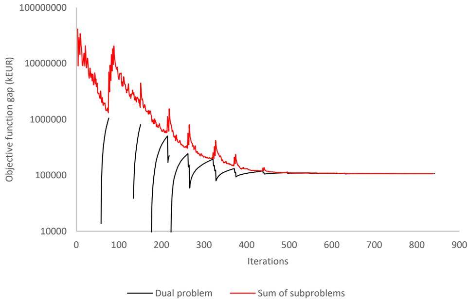
**Figure 40: The evolution of the convergence gap of the LR solution process for parameter values from configuration 3.**
