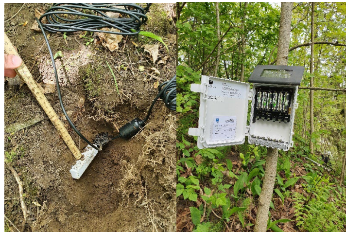
Figure 6: a) installation of sensors at depth of 0.1m; b) Datalogger.
