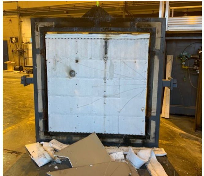
Figure 5 Result after small-scale test with inlaid mistakes and damages (12, 5 mm gypsum plate type A, 10 minutes)
