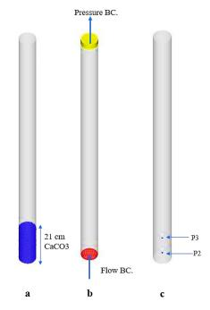
Figure 5. Initial condition (a), boundary condition (b) and transient points (c)
