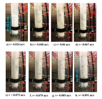
Figure 2. Snapshots from experimental tests with different superficial gas velocities
