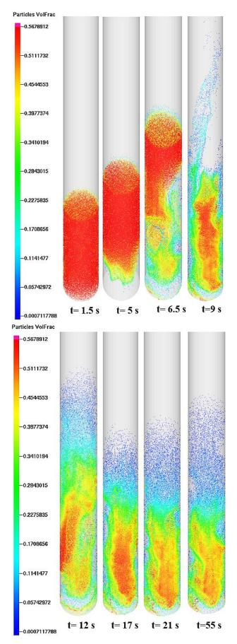
Figure 6. Simulation results of particle volume fraction of limestone
