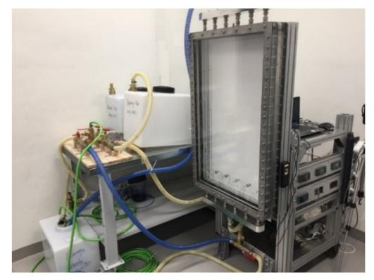
Figure 3. Experimental setup for performing the tests in the eccentric Hele–Shaw cell.
