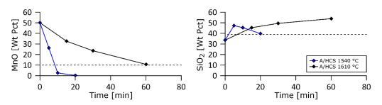
**Figure 5.** MnO and SiO<sub>2</sub> weight fractions in the slag as a function of time for the A/HCS charge at 1540 and 1610  $^{\circ}$ C.
