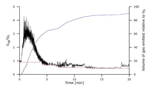
**Figure 13.** Droplet dimensions for the experiment A/HCS-1610-20. Volume of the slag + gas  $V_{sg}/V_0$  is in black, volume of the slag  $V_s/V_0$  is in red, and the volume of the gas emitted relative to  $V_0$  is in blue.
