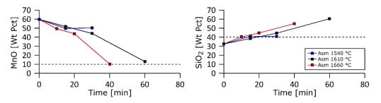
**Figure 4.** MnO and SiO<sub>2</sub> weight fractions in the slag as a function of time for the Asm charge at 1540, 1610, and 1660  $^{\circ}$ C.
