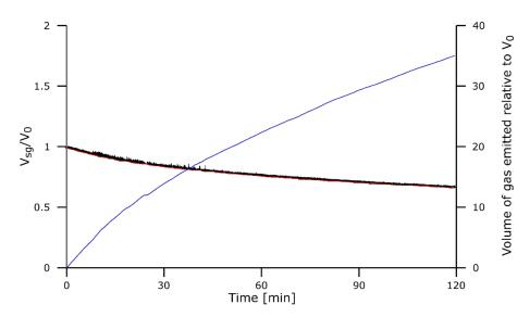
**Figure 14.** Droplet dimensions for the experiment Com-1610-120. Volume of the slag + gas  $V_{sg}/V_0$  is in black, the volume of the slag  $V_s/V_0$  is in red, and the volume of the gas emitted relative to  $V_0$  is in blue.
