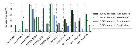
**Figure 16.** Fractions of MnO and SiO<sub>2</sub> reduced for similar experiments using a tube furnace (data adapted from Canaguier et al. [4]) and a sessile drop (present work).
