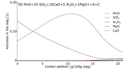
**Figure 17.** Evolution of the activities in a silicomanganese slag at 1650 °C with the addition of carbon. Calculated using FactSage 8.0 [15].
