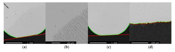
**Figure 10.** EPMA images of the reacted slag sample and graphite substrate, respectively, contoured by green and red lines: (a) Com sample reacted at 1610 °C for 30 min; (b) close-up of the interface on the Com sample reacted at 1610 °C for 30 min; (c) Com + S sample reacted at 1610 °C for 10 min; (d) slag/graphite interface of the Com + S sample reacted at 1610 °C for 10 min.
