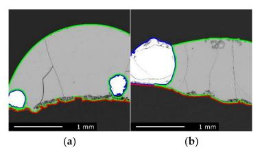
**Figure 9.** EPMA images of the reacted A/HCS slag sample, graphite substrate, and metal phase, respectively, contoured by green, red, and blue lines: (**a**) sample reacted at 1540 °C for 30 min; (**b**) sample reacted at 1610 °C for 10 min.
