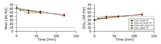
**Figure 6.** MnO and SiO<sub>2</sub> weight fractions in the slag as a function of time for the Com, Com + S, and Com + 2S charges at 1610 and 1660  $^{\circ}$ C.
