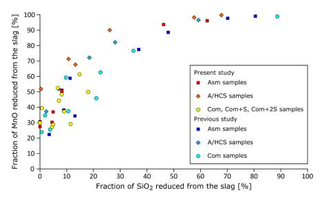
**Figure 3.** Fraction of MnO and SiO<sub>2</sub> reduced from SiMn slags. The original data from the present study were colored in cold tones, while the warm colored markers show data from previous work [4]. The data ranged from 1510 to 1660  $^{\circ}$ C.
