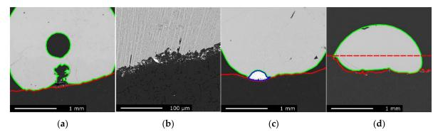
**Figure 7.** EPMA images of the reacted Asm slag sample, graphite substrate, and metal phase, respectively, contoured by green, red, and blue lines: (**a**) sample reacted at 1540 °C for 15 min; (**b**) slag/graphite interface of the sample reacted at 1610 °C for 15 min; (**c**) sample reacted at 1610 °C for 15 min; (**d**) sample reacted at 1660 °C for 40 min. The red, dashed line is an estimate of the initial substrate's surface.
