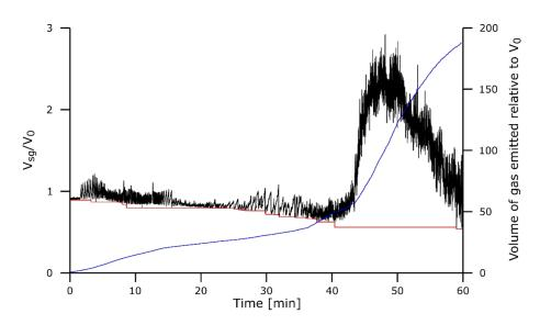
**Figure 11.** Droplet dimensions for the experiment Asm-1610-60. Volume of the slag + gas  $V_{sg}/V_0$  is in black, the volume of slag  $V_s/V_0$  is in red, and the volume of the gas emitted relative to  $V_0$  is in blue.
