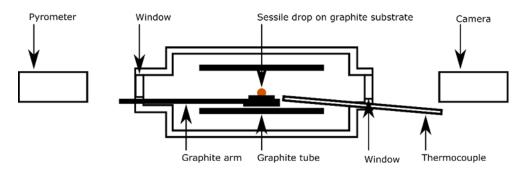
Figure 1. Schematics of the sessile drop furnace.
