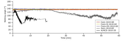
Figure 15. Wetting angle for each charge type of the study upon reaction at 1610 °C.
