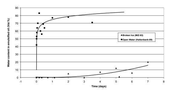
Figure 4.2 - Example on variations in water content for crude oil as a function of weathering in ice covered and open water.
