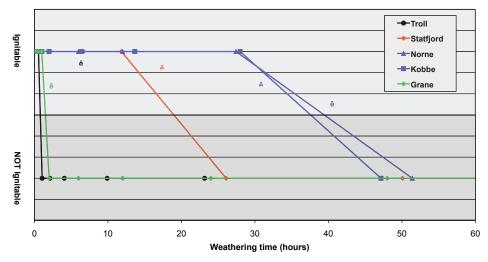
Figure 5.2 - Ignitability measured with the laboratory burning cell as a function of weathering time for the five different oil types used in this study. All were measured at 50% ice coverage.
