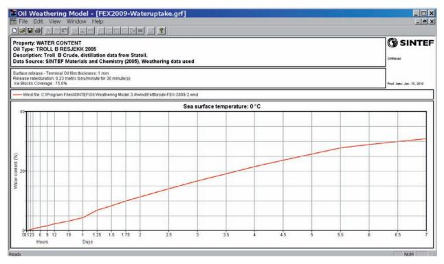
Figure 4.4 - Water content predicted with the SINTEF Oil Weathering Model improved for predicting oil weathering in ice. Predictions are for Troll B with ice conditions and wind from the field experiment in May 2009 (FEX2009).
