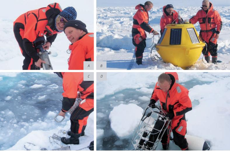
Fig. 9.2 - Examples from FEX 2009 measurment program A) Seaguard - current measurements B) Mini Seawatch – waves in ice field C) Deployment of SPMD D) Deployment of KISP
