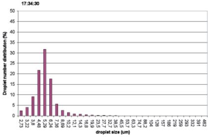
Figure 6.3 - Droplet size measurements document that the oil is broken down into small particles (5-30 um) with extremely low rising velocity
