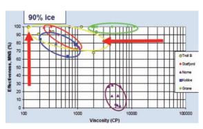
Figure 6.1 - Weathering of oil vs. dispersibility and ice coverage. The figure shows that the "clusters" of the viscosity range for the different oils are generally lower when weathered in high ice conditions compared to no ice, and that this results in a higher dispersant effectiveness for some of the oils.
