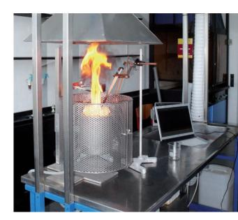
Figure 5.1 - The new laboratory burning cell during initial testing
