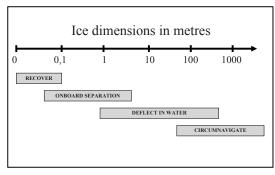
Figure 7.1 - Main ice processing principles roughly related to ice dimensions (metres)
