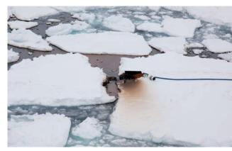
The oil spreads in between the ice floes and will follow the movement of the ice
