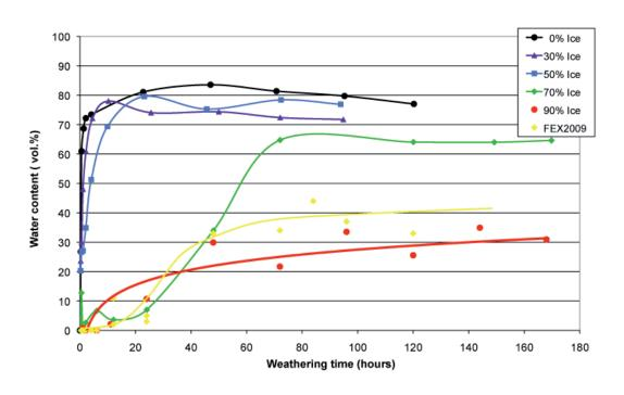
Figure 4.3 - Water content (vol.% water in emulsion) for the Troll B crude for different ice conditions (0, 30, 50, 70 and 90% ice coverage) as a function of weathering time in the mesoscale flume. The water uptake measured during the field trial in May 2009 (FEX2009) is also plotted in the figure.
