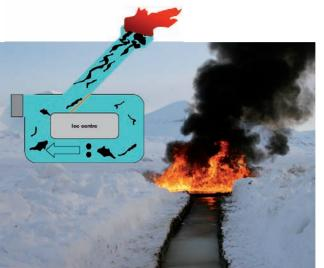
Figure 53 - In-situ burning of weathered oil. The system consisting of a burning basin connected to the weathering basin with a channel (see earlier figure) in operation.
