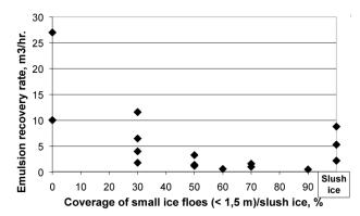
Figure 7.3 -Calculated recovery rates as a function of increased coverage of small ice floes
