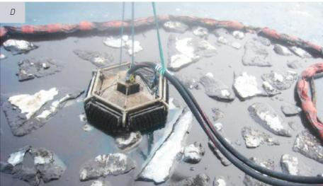
Figur 7.2 Testing of skimmers in laboratory and field experiments. A) Lamor LRB 150 Brush drum skimmer (SINTEF Sealab)
