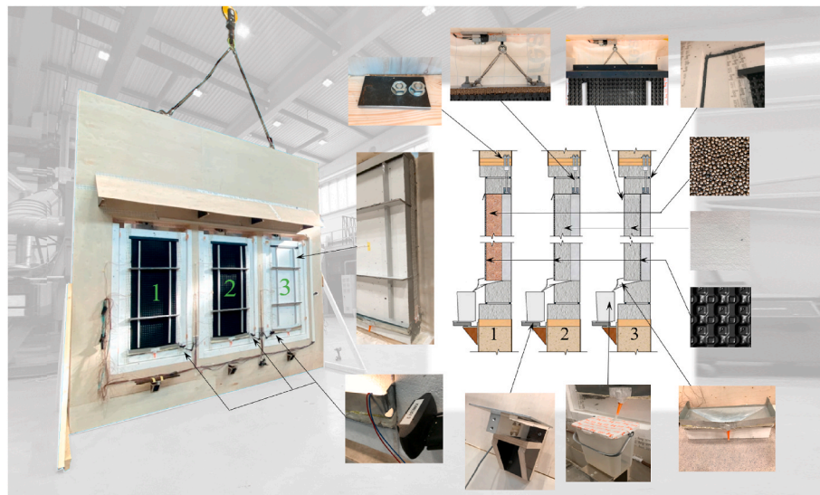
Fig. 5. Details of the weighed wall segments and wooden frame. Enlarged versions of the photographs and a detailed explanation of the compositions are presented in Ref. [38].
