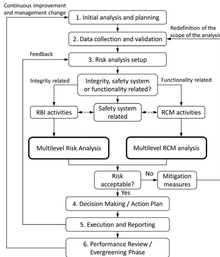
**Figure 3.** Framework of RBIM procedure within the overall management system (adapted from [14]).
