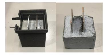
Figure 1. Photography of sample in the 3D printed mold and sample removed from the mold.
