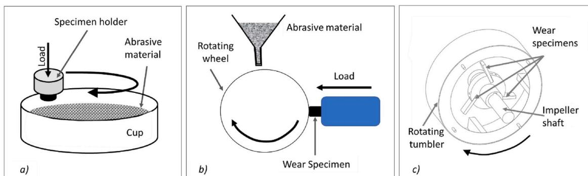
Fig. 1. Schematic representation of kinematics systems in selected laboratory wear tests used for hard materials: a) crushing pin-on-disc test, b) rotating wheel test, and c) impeller-tumbler impact abrasive test.
