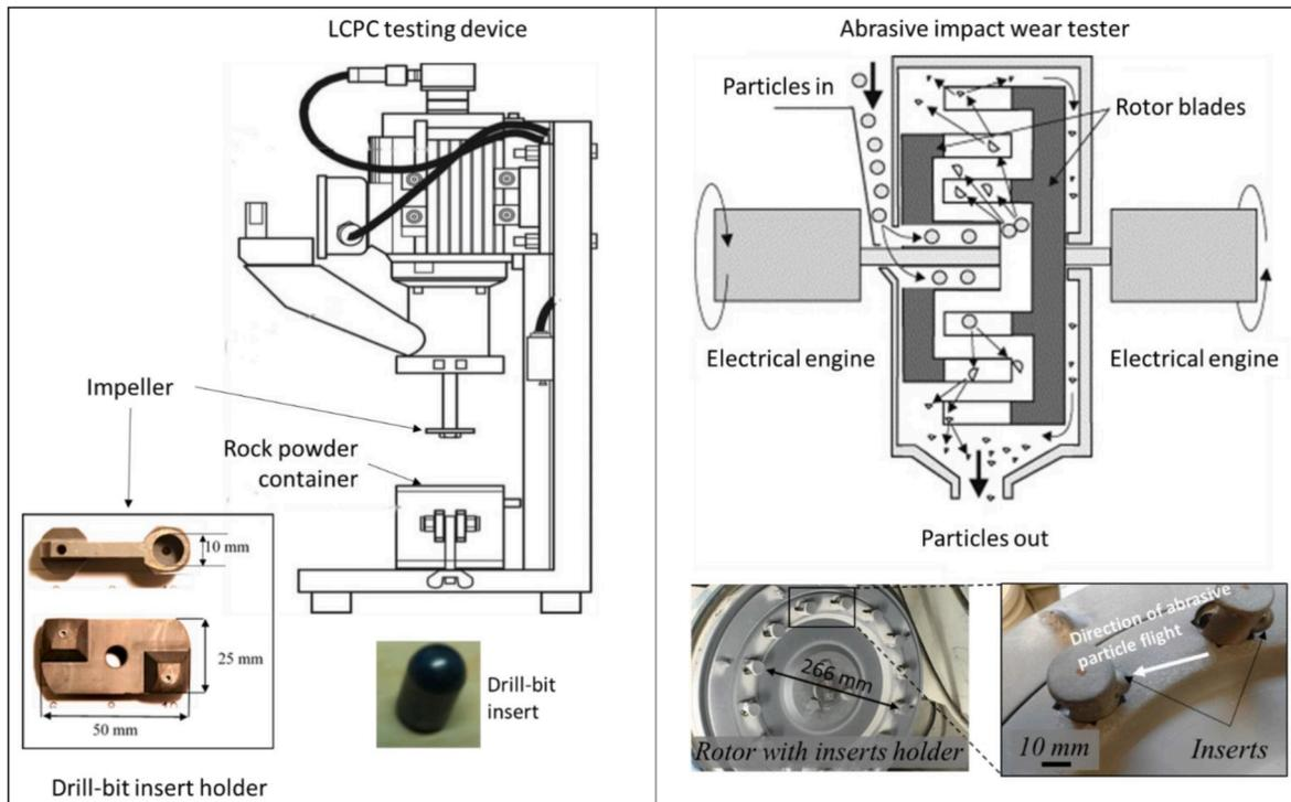
Fig. 3. Schematic illustration of the LCPC testing device (left side) and disintegrator impact wear tester (right side) with the corresponding inserts holders.
