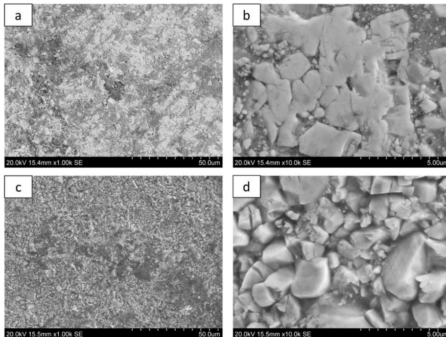
Fig. 7. Secondary-electron SEM images of standard WC-Co insert before (a and b) and after 20 min (c and d) of LCPC abrasive impact wear test (see Fig. 5).
