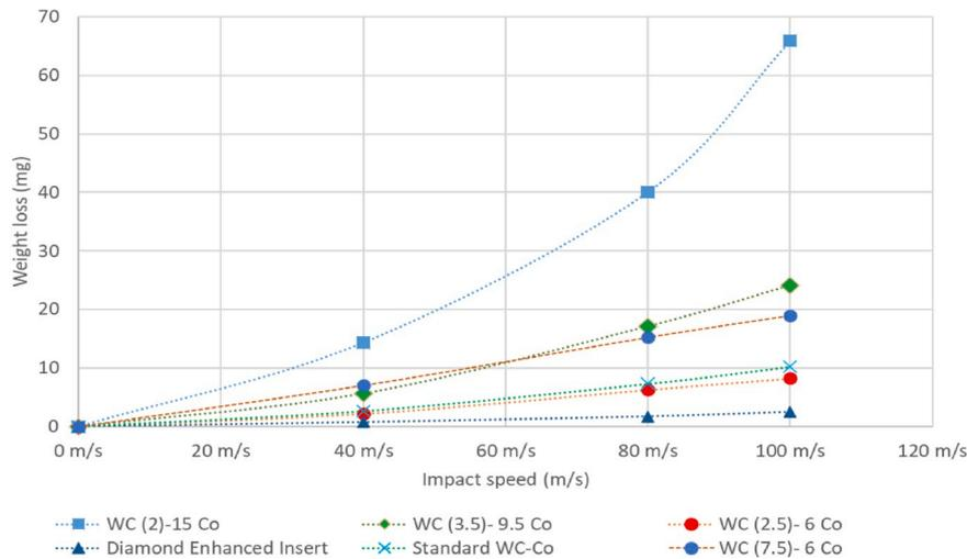
Fig. 6. Effect of impact speed on weight loss measurements by disintegrator abrasive impact wear tests.
