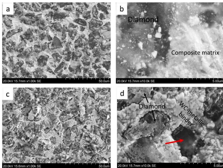
**Fig. 8.** Secondary-electron SEM images of diamond-enhanced material before (a–b) and after (c–d) 20 min of LCPC abrasive impact wear testing (see Fig. 5). The diamond particles appear dark, while the WC- metallic binder is bright. A hole where a diamond particle might have been removed during testing is indicated by a red arrow in (d). (For interpretation of the references to colour in this figure legend, the reader is referred to the Web version of this article.)
