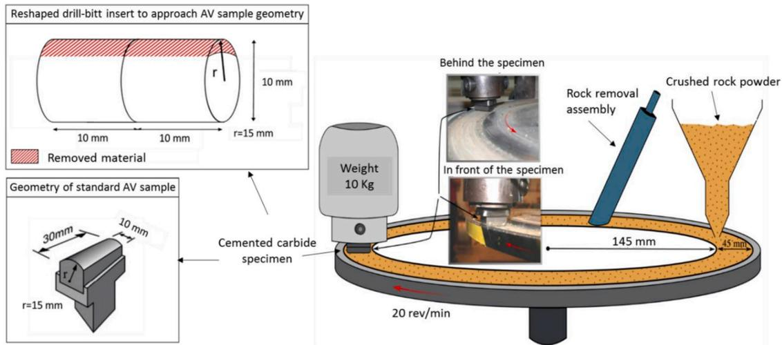
Fig. 2. Schematic illustration of the abrasive sliding wear test and the geometries of reshaped insert specimen compared to the standard AV test specimen.
