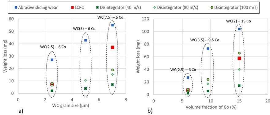
Fig. 4. Influences of WC grain size (a) and Co volume fraction (b) on the weight loss measurements by abrasive sliding wear tests, LCPC abrasive impact wear tests and disintegrator abrasive impact wear tests at 40 m/s, 80 m/s and 100 m/s.
