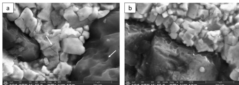
**Fig. 10.** Secondary-electron SEM images of diamond-enhanced composite after LCPC testing. In (a), white arrows indicate a cracked WC grain, and a faceted hole in a diamond particle.
