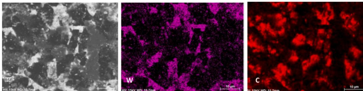
**Fig. 9.** Backscattered-electron SEM image and EDX (energy-dispersive x-ray spectroscopy) maps of untested diamond-enhanced insert. The carbon map (right side image) shows the location of the diamond while the tungsten map (middle image) reveals the WC grains in the composite matrix.
