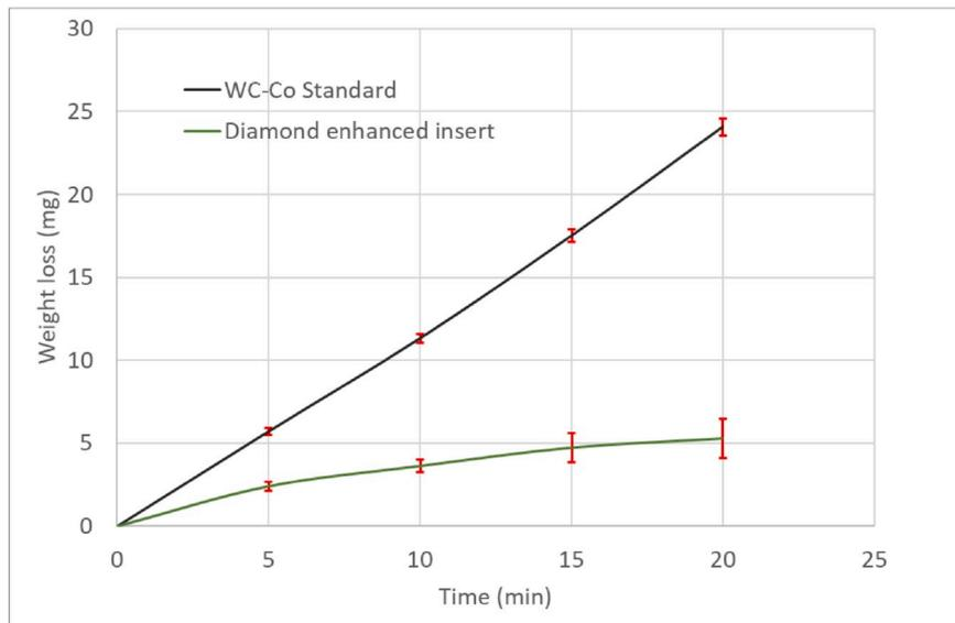
Fig. 5. Time dependent measurements of DEI by LCPC abrasive impact wear test compared to time dependent measurements of standard WC-Co insert. The error bars represent measurements deviation around the mean values.
