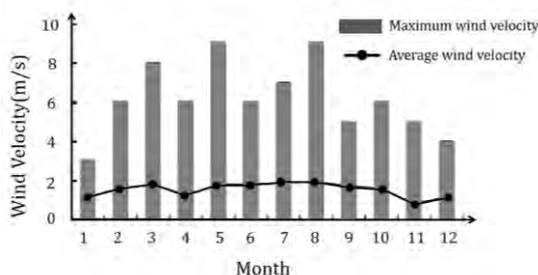
Figure 5. Wind velocity distribution of typical year
