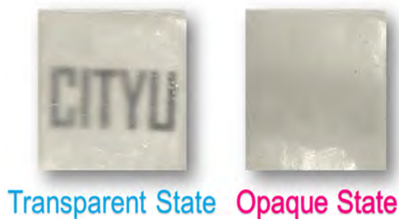
Figure 2. (c) Transparency and opacity of the HWC at the transparent state and opaque state.
