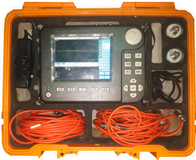
Fig. 2. ZBL-U520 non-metal pulse velocity test equipment.
