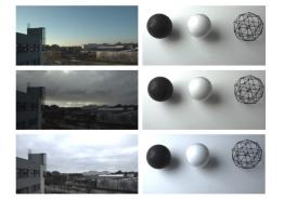
Figure 4. Different sky conditions, from the top and down referring to the daylight inflow with respectively CIE sky types 13, 3 and 8 and to the right photo illustrating how the different daylight situations affect light modelling qualities of the spheres. Photo: Mihkel Pajuste.
