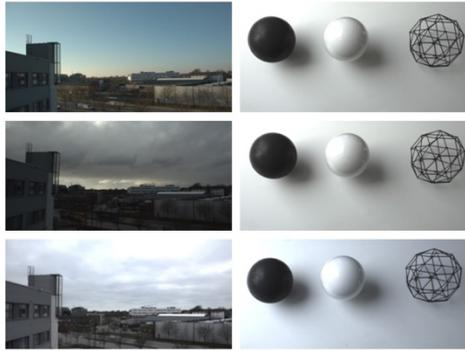
Figure 4. Different sky conditions, from the top and down referring to the daylight inflow with respectively CIE sky types 13, 3 and 8 and to the right photo illustrating how the different daylight situations affect light modelling qualities of the spheres. Photo: Mihkel Pajuste.
