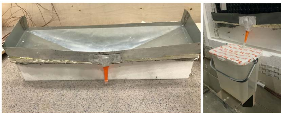
Figure 5.10: Metal fittings and water tanks mounted underneath the wall segments.
