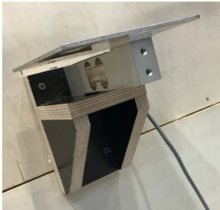
Figure 5.9: The load cells weighing the condensed water were screwed onto brackets made of plywood.
