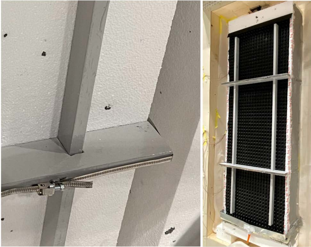
Figure 5.6: Thermal insulation and dimpled membrane gently pressed against the concrete segments and held in place by means of frames and band-hose clamps.
