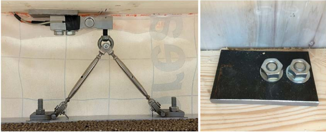
Figure 5.8: Suspended load cell and attachment details (left), and steel plate mounted above and below the attachment of the load cells (right).
