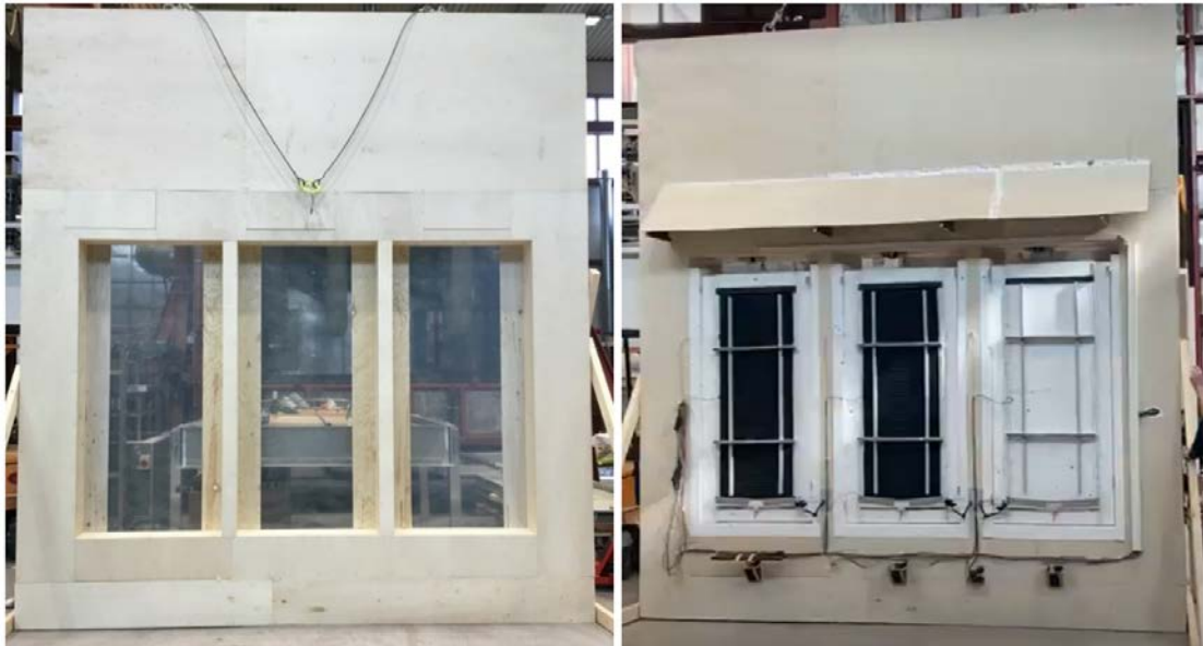
Figure 5.4: Wooden frame (left) and roof overhang (right)
