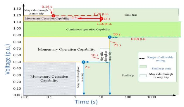
Figure 3.5 - DER response to abnormal voltages and voltage ride-through requirements for DER of abnormal operating performance Category III. [2]
