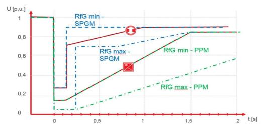
Figure 3.11 - Voltage-time-profile for generation units of type B for synchronous (SPGM) and power park modules (PPM). Maximum and minimum limits in NC-RfG illustrated for synchronous production units (blue) and power-park units (green) Ref Statnett Reviewed RfG NC. [4]
