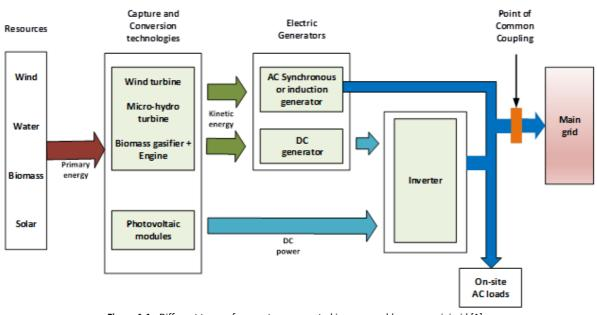
Figure 1.1 - Different types of generators connected in a renewable power minigrid [1]
