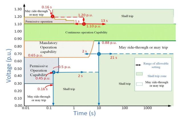
Figure 3.4 - DER response to abnormal voltages and voltage ride-through requirements for DER of abnormal operating performance Category II. [2]
