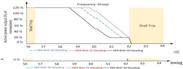
describes the frequency (ride-through) response requirement of DER, while Figure 3.7 shows an example case of Frequency droop characteristics under varying frequencies, as specified.
