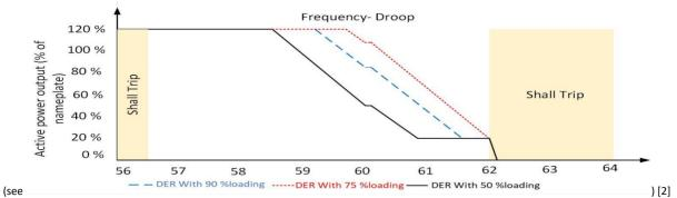
Adjustable underfrequency trip settings shall be coordinated with Area EPS operations.
