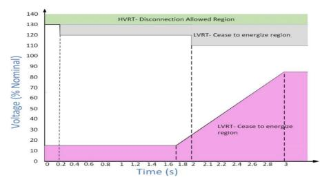
Figure 3.13 - Voltage ride through limit (X-axis values are as per CEA standard mentioned earlier). [7]
