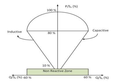
P: Active power; Q: Reactive Power; Sn: Maximum apparent Power of the inverter
