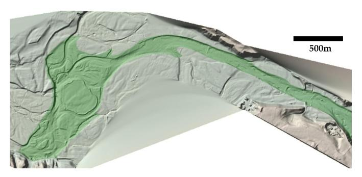
**Figure 9.** Bathymetry for a 5 km reach in river Nea. The bathymetry was calculated using an adjusted regional model setup on an aerial image combined with LIDAR data in dry areas. The green color outlines are the main river course which runs from right to left.
