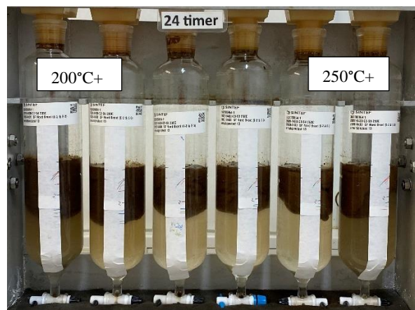
Figure 5-1 Rotating cylinders of water-in-oil (w/o) emulsions of SF Nord Brent (E-2&E-3) after 24 hours at 13 °C. The figures show from left to right emulsions prepared from the residues of 150°C+, 200°C+ and 250°C+.
