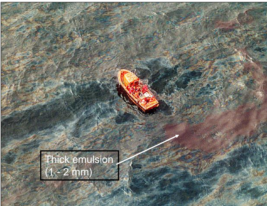
Figure A-11 Surface oil slick (initial thickness > 200 \mu\text{m} ) from the experimental deep-water release DeepSpill in 2000. Surface oil is emulsifying similar to an oil slick from a surface batch release (from Leirvik et al., 2011).
