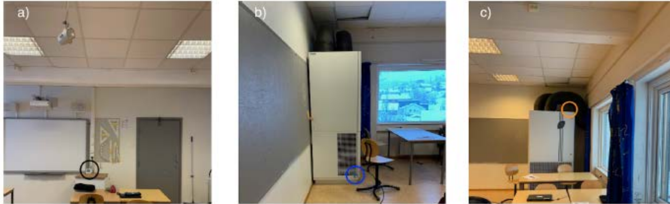
Figure 3.9: Location of placement of sensors in classroom 104. a) Sensor, measuring air quality b) Sensor measuring temperature of supply-air, and c) Sensor measuring temperature of extract-air
