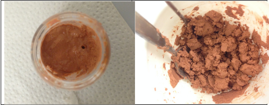
Figure 3: Calcined clay 1 paste mix without plasticizer (right) and calcined clay 2 mix with plasticizer and 10.8 % increased amount of accelerator (left). Both pastes had w/b = 0.70 .
