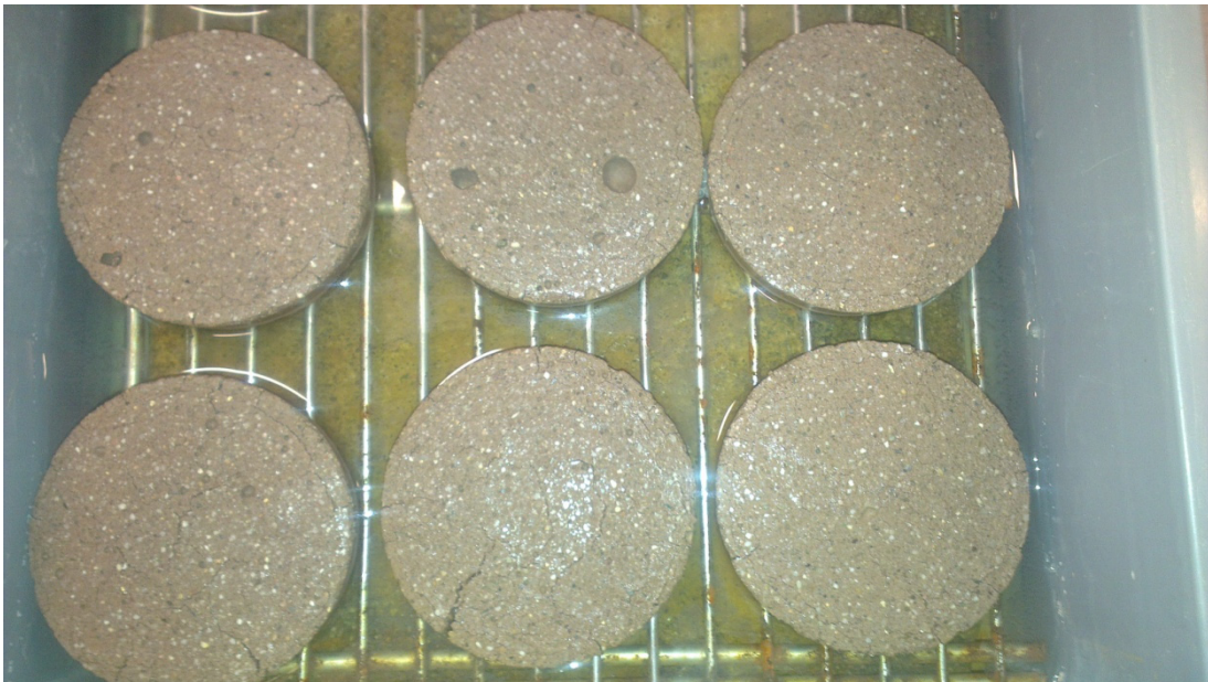
Figure 7: Mortar discs of Mix 8 in the capillary suction set-up. Note that the discs are swollen to an extent that cracks are induced.
