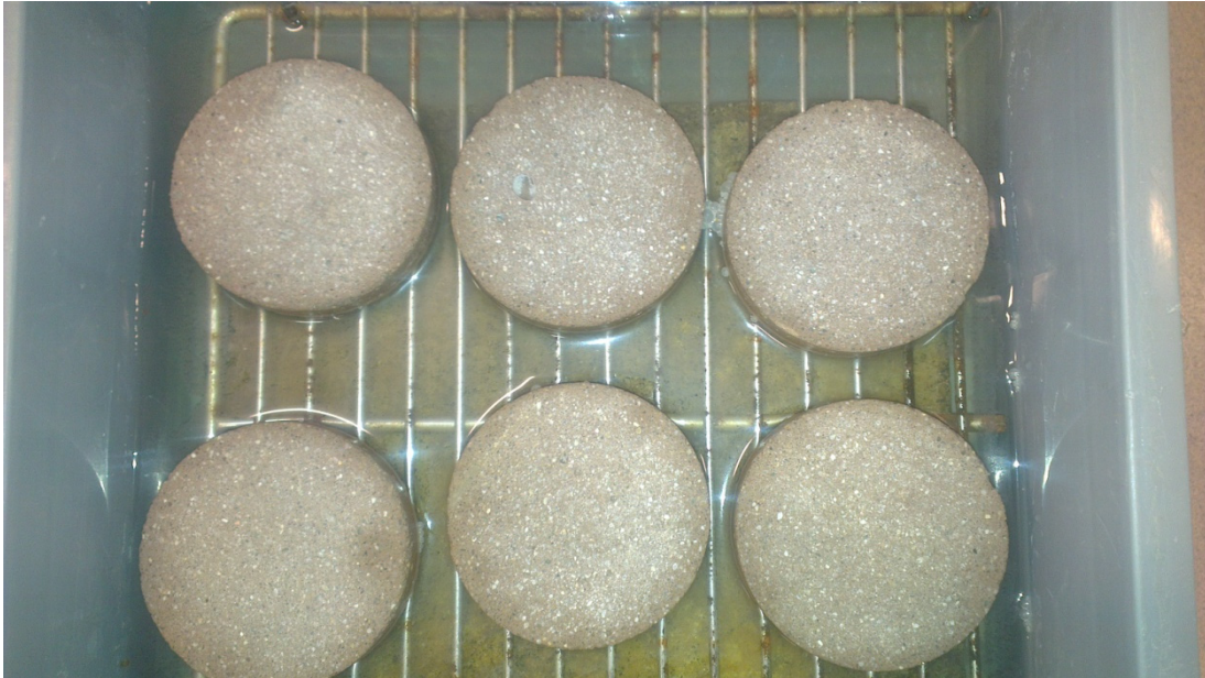
Figure 6: Mortar discs of Mix 9 in the capillary suction set-up.
