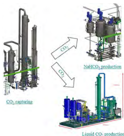
Figure 2. Schematics of Twence's CO 2 capture pilot plant
