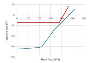
Figure 3: Composite curve for heat integration
