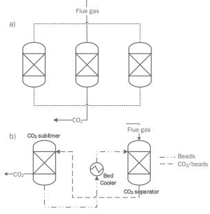
Figure 2: Schematic representation of cryogenic CO<sub>2</sub> capture unit: a) fixed packed columns and b) moving packed beds
