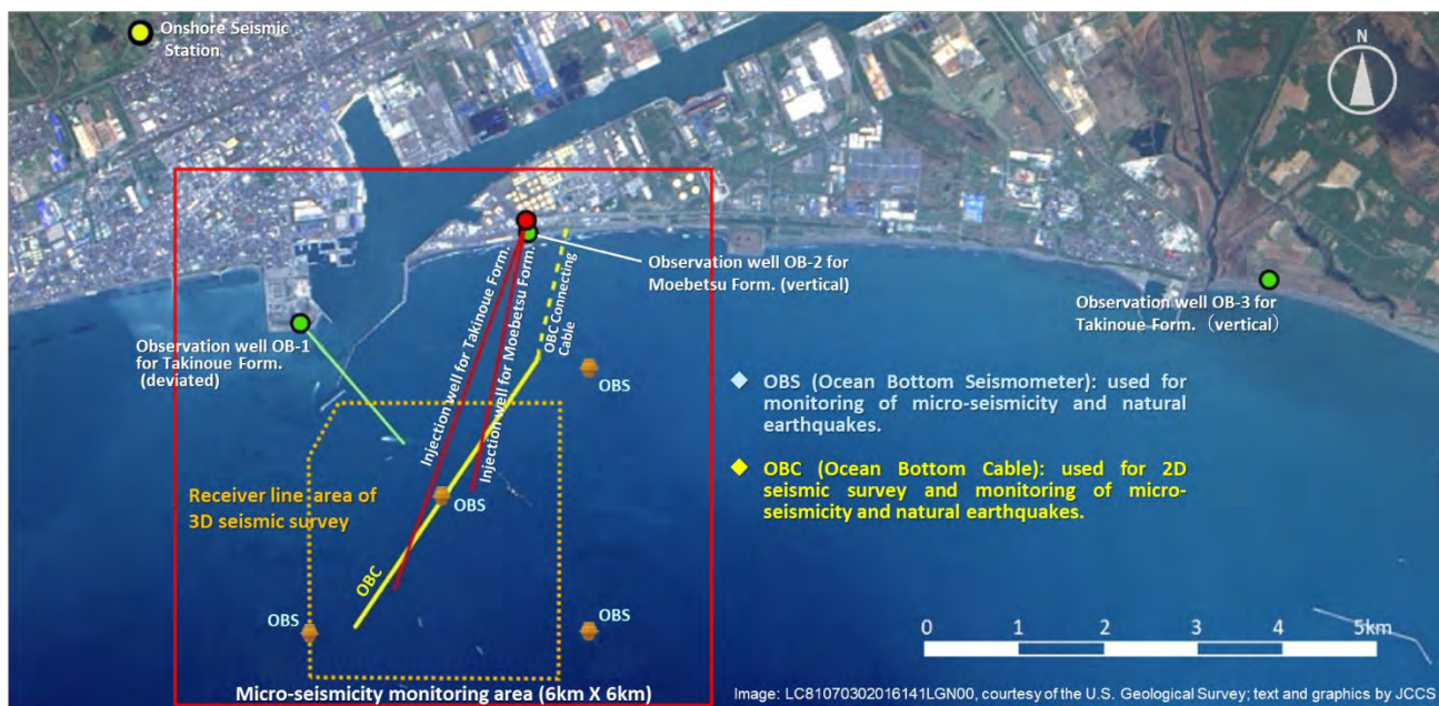
Figure 7: Layout of monitoring facilities
