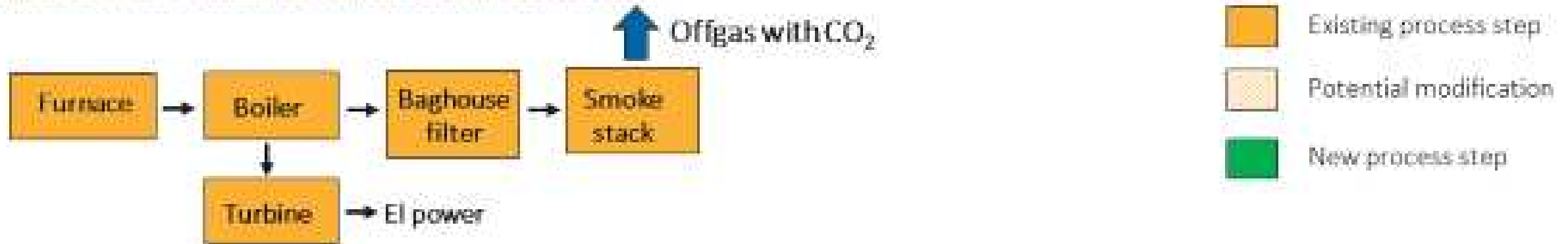
FURNACE OFFGAS PROCESS WITH ENERGY RECOVERY
