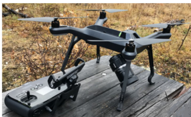
Figure 4. Data acquisition equipment: unmanned aerial vehicle 3DR Site scan.
