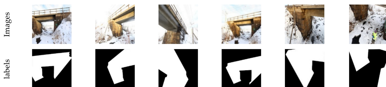
Figure 6. Examples of the prepared dataset for bridge component detection and their corresponding labels.
