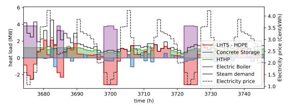
Figure 16. Cutout of the thermal storage and steam generator loads, steam demand and electricity price profiles for Case 2.
