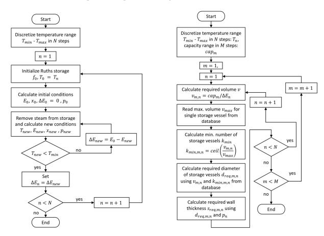
Figure 2. Ruths steam accumulator: calculation of vessel capacities (left) and calculation of storage parameters (right).
