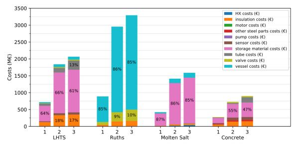
**Figure 9.** Cost structure for all selected TES technologies for Case 1 for three capacity (Cap.)/heat load (HL) scenarios—1: Low Cap./Low HL, 2: High Cap./Low HL, 3: High Cap./High HL.
