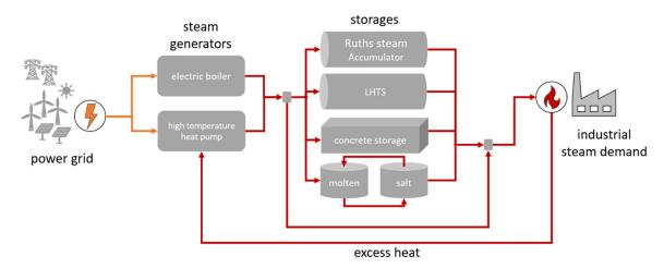
**Figure 1.** Schematic of the electricity-driven steam supply system considered within this work, showing the nodes and connectors considered in the model.
