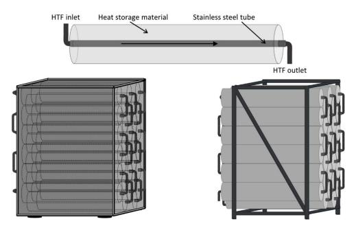
**Figure 3.** Schematic drawings of the tube surrounded by heat storage material for both LHTS and concrete storage (**top**), the LHTS system (**left**) and the concrete storage system (**right**) considered in this work. Both TES systems are represented without thermal insulation material.
