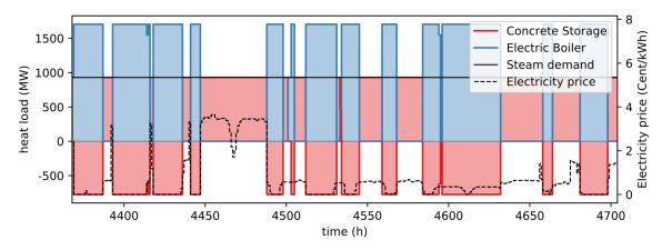
Figure 12. Storage and steam generator loads, steam demand and electricity price profiles for Case 1 during wet season.
