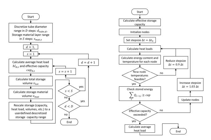
**Figure 4.** Flow-charts for the calculation of storage parameters for LHTS and concrete storages (**left**) and for the calculation of average heat loads (**right**).
