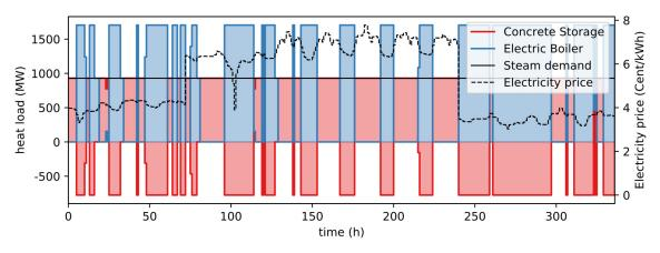
Figure 11. Storage and steam generator loads, steam demand and electricity price profiles for Case 1 during dry season.
