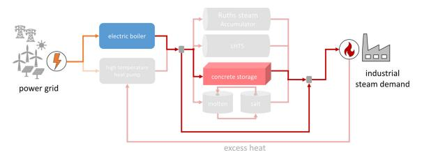
Figure 10. Optimal power-to-heat (P2H) system for Case 1.
