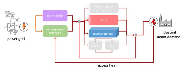
Figure 15. Optimal P2H system for Case 2 including electric boilers, high-temperature heat pumps, LHTS and concrete storage.
