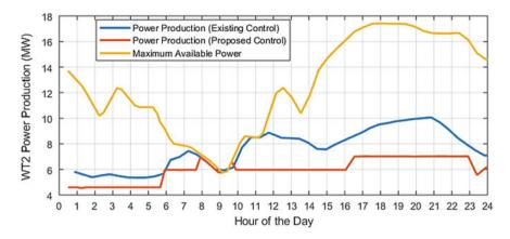
Fig. 6 Comparison of WT2 Power Production profiles
