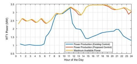
Fig. 5 Comparison of WT1 Power Production profiles
