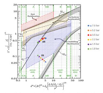
Fig. 14. Fluidization regime of AR (circle) and FR (triangle) under different pressure, the operating condition taken from Fig. 13.
