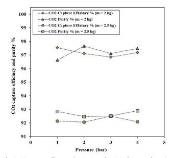
Fig. 8.  $CO_2$  capture efficacy and purity % as function of pressure for various solids inventory (2 and 2.5 kg),  $U_{AR} = 0.53$  m/s, case (2,5,8,11,15) compared with case (19,20,21,25).
