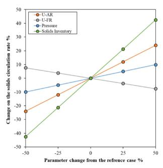
Fig. 12. Sensitivity analysis for the effects of the various independent variables on the solids circulation rate.
