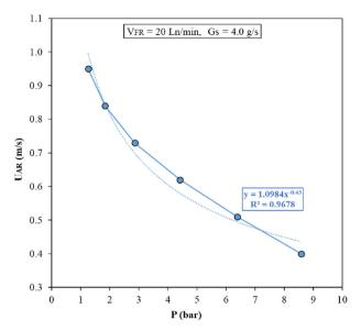
Fig. 13. Predicted  $U_{AR}$  as function of pressure at a constant solids circulation rate and thermal power of the fuel.
