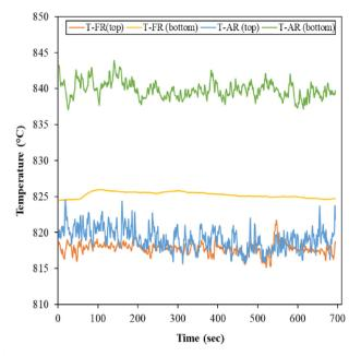
**Fig. 15.** Temperature profile in FR and AR during an autothermal PCLC test, P = 3 bar, AR flowrate = 120 Nl/min, FR flowrate = 20 Nl/min, solids inventory = 2.5 kg (case-8).
