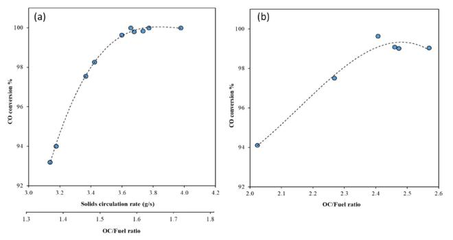
Fig. 10. a) CO conversion with different solids circulation rate and OC/fuel ratio, (solids inventory = 2.5 kg), b) CO conversion with different OC/fuel ratio, (solids inventory = 2.0 kg).
