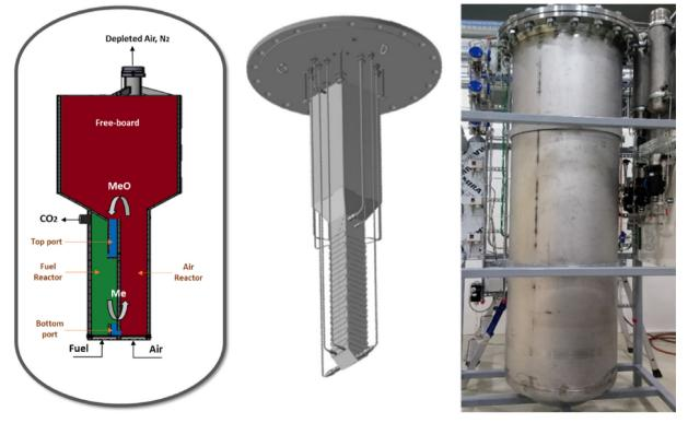
Fig. 1. From left to right; a simplified scheme of the ICR design, CAD drawing of the ICR unit, and the ICR unit under operation inside the shell.
