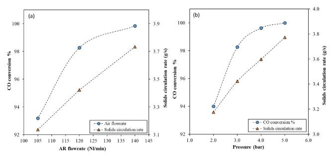
Fig. 9. a) Effect of AR flowrate on CO conversion and solids circulation rate, (Pressure = 3 bar). b) Effect of pressure on CO conversion and solids circulation rate, (FR specific inventory = 393 kg/MW).
