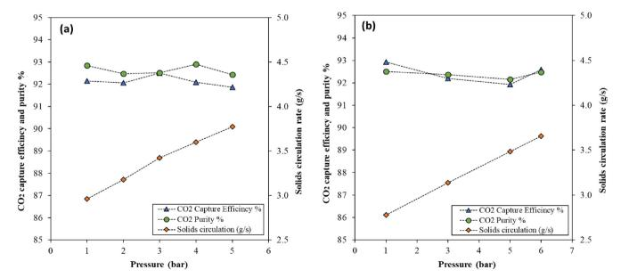
Fig. 5. Solids circulation rate and CO<sub>2</sub> capture efficiency and purity % as function of pressure, a)  $U_{AR} = 0.53$  m/s, case (2,5,8,11,15), b)  $U_{AR} = 0.46$  m/s, case (1,9,17,18).
