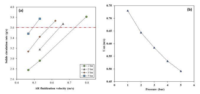
Fig. 6. a) Solids circulation rate as function of air fluidization velocity in AR at various pressure, b) the estimated air fluidization velocity in AR as function of pressure that keep solids circulation rate constant at 3.6 g/s.
