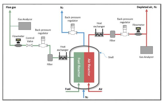
Fig. 2. A simplified illustration of the ICR auxiliary components.
