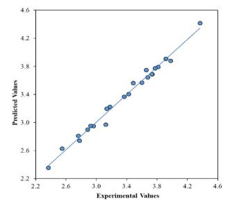
Fig. 11. Reconciliation plot between predicted and experimental solids circulation rate.
