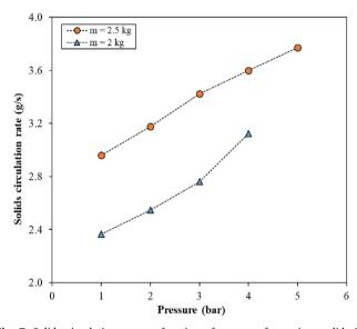
Fig. 7. Solids circulation rate as function of pressure for various solids inventories (2 and 2.5 kg),  $U_{AR} = 0.53$  m/s, case (2,5,8,11,15) compared with case (19,20,21,25).
