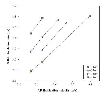
Fig. 4. Solids circulation rate as function of air fluidization velocity in AR at various pressure.
