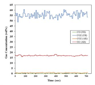
Fig. 3. Gas product concentration measured at the FR and AR outlet during PCLC tests (case-11).
