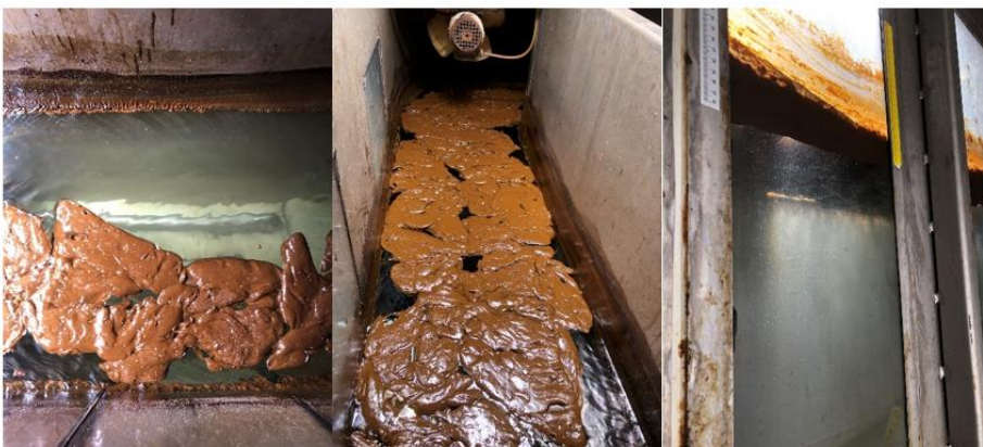
Figure 5-11 Surface at 168 hours (7 days). Water content: 80 vol.%. Viscosity: 22 083 mPa.s. Images taken prior to dispersant application.
