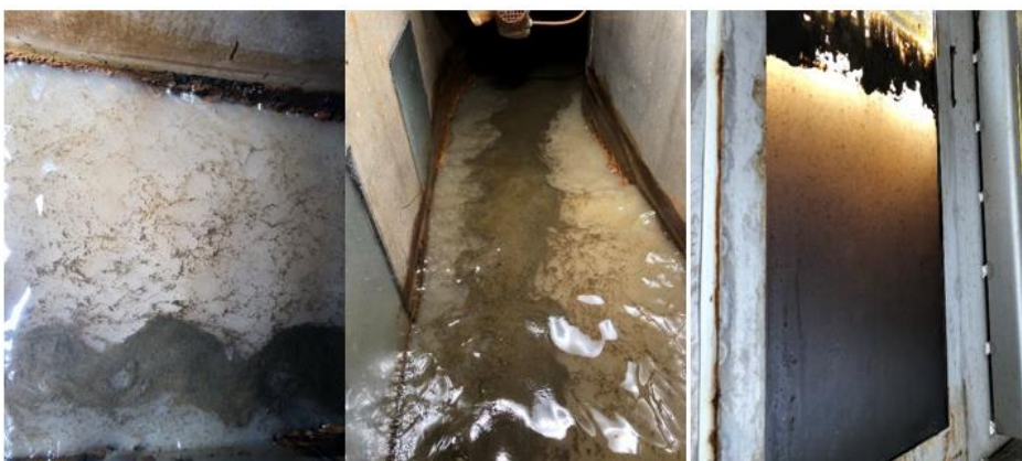
Figure 5-6 Surface 10 minutes after 4. round of application of dispersant on IM-5 Wakashio at 2 °C. The structure in the emulsion is broken and the effect of the dispersant is apparent. About 49 % of the original amount of oil was dispersed into the water phase.
