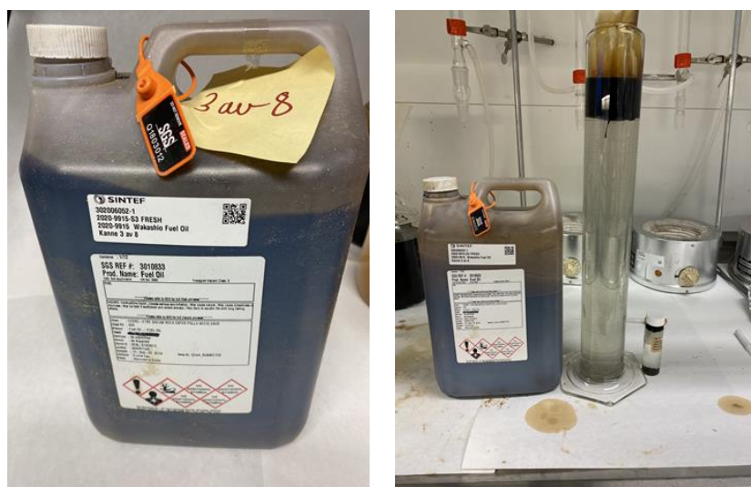
Figure 4-1 Left: 1 of the 8 cans with IM-5 Wakashio. Right: Free-water, approx.1 litre of seawater, drained off from one of the cans.
