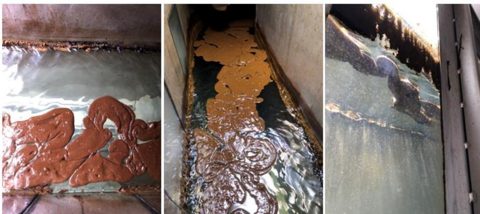
Figure 5-5 Surface at 168 hours (7 days) of IM-5 Wakashio at 2 °C. Water content: 66 vol.%. Viscosity: 39 960 mPa.s. Images taken prior to dispersant application.
