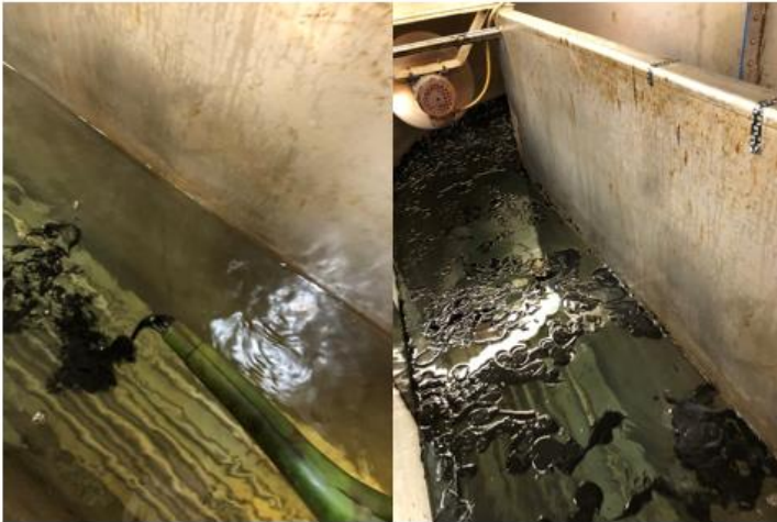
Figure 5-4 Application of IM-5 Wakashio onto the water surface at 2 °C.
