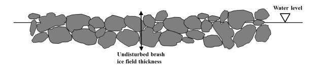
Fig. 1. Typical cross section of brash-ice field
