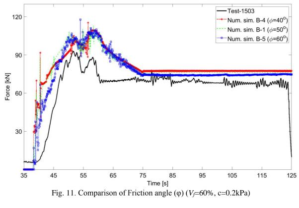
The cohesion values were altered to examine their influence with respect to the measured force time history, see Fig. 12 and Fig. 13. The simulation series "A" has 70 % void fraction and "B" has 60% void fraction. In simulations A-1, A-2 and A-3 cohesion values of 0.2kPa, 0.05kPa and 1kPa were used respectively.
