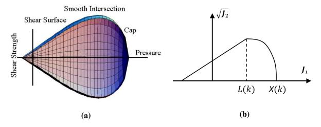
Fig. 8. General shape of the CSCM model yield surface in meridional plane (from Murray et al. (2007)). (b) Single smooth cap failure function (from Schwer and Murray (1994))
