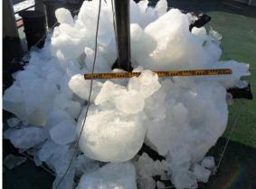
(b) Ice blocks collected by the collector after the test
