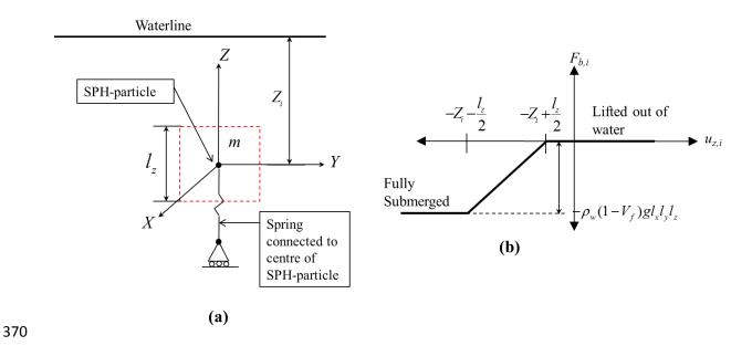
Fig. 7. (a) Mass-spring-dashpot model for SPH Particle. (b) The force vs. displacement
