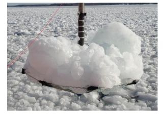
(a) Plug formed after collector is completely removed from the water and is hanging in the air
