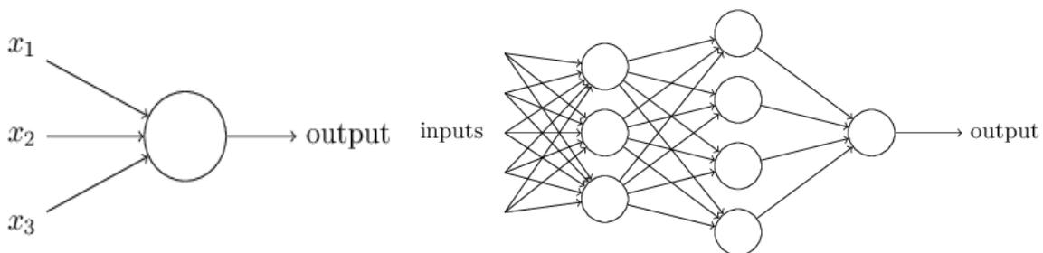
**Figure 5.3** Illustration of a single perceptron (*left*) as well as a simple multilayer perceptron (*right*). The network on the right is a feedforward neural network with two hidden layers. Both illustrations are taken from chapter 1 in [57]
