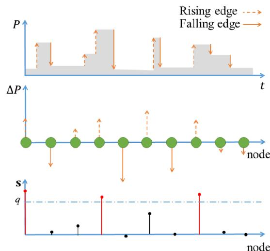
**Figure 5.1 Generation of a graph representation of power consumption data**
